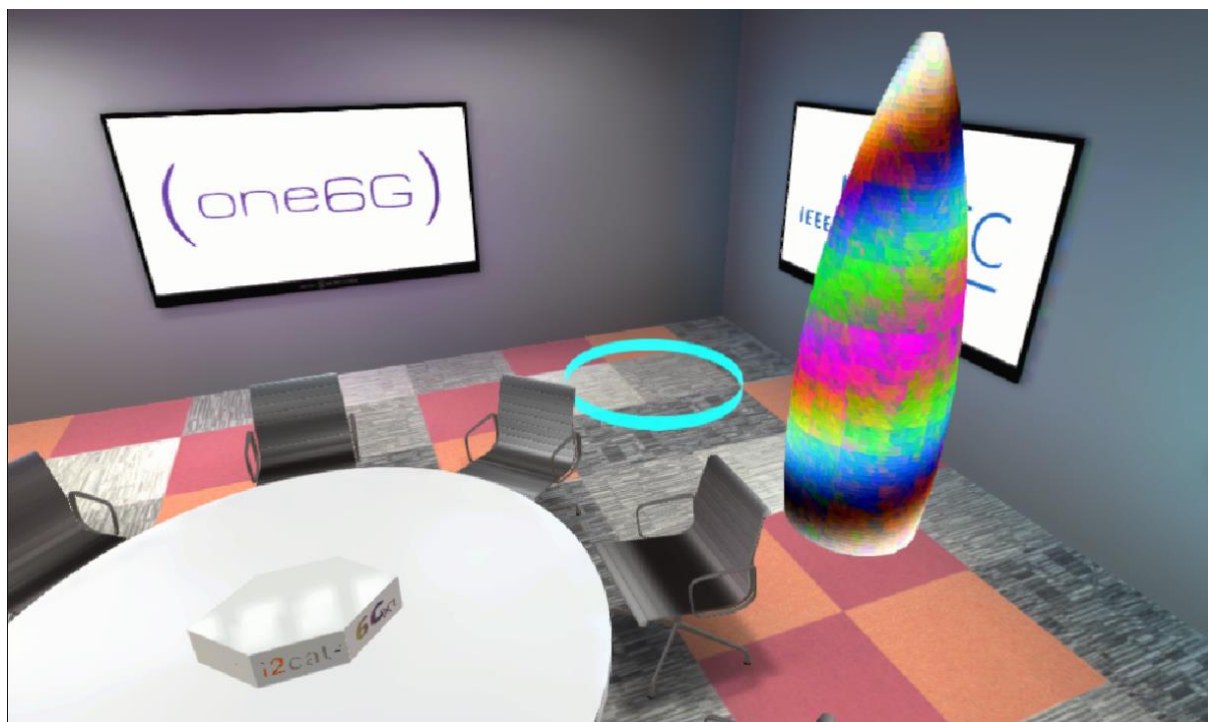
Figure 10. Remote Renderer running as a standalone application with a synthetic point cloud in the VR scene.
