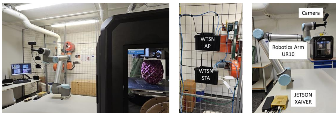
Figure 16: Robot arm with Camera for 3D printer Surveillance.
