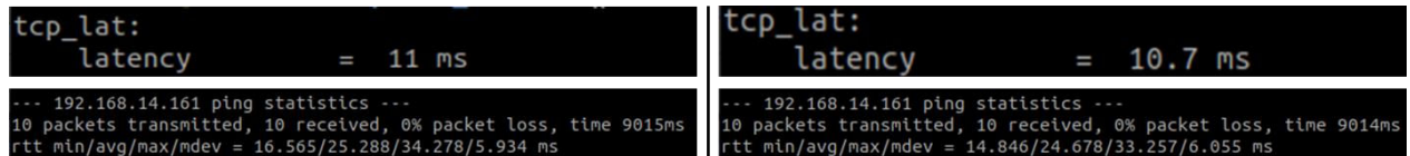
Figure 61: Network latency and RTT for test run 1 (left) and 2 (right).
