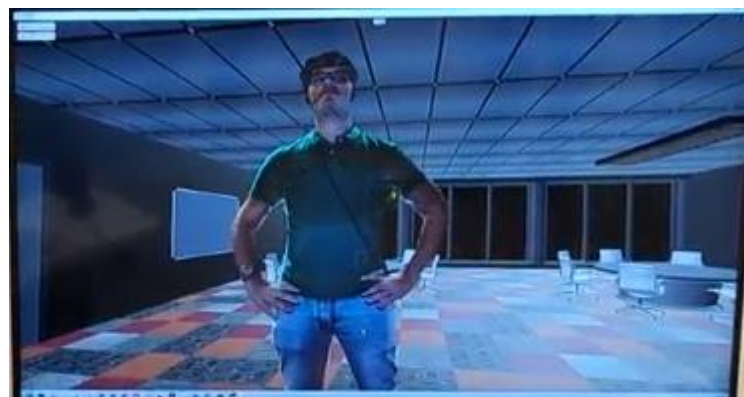
Figure 34: Hologram received at Holo Client 2, representing the real-time 3D person representation captured and reconstructed by Holo Client 1 and sent to Holo Client 2 via the 5G network.
