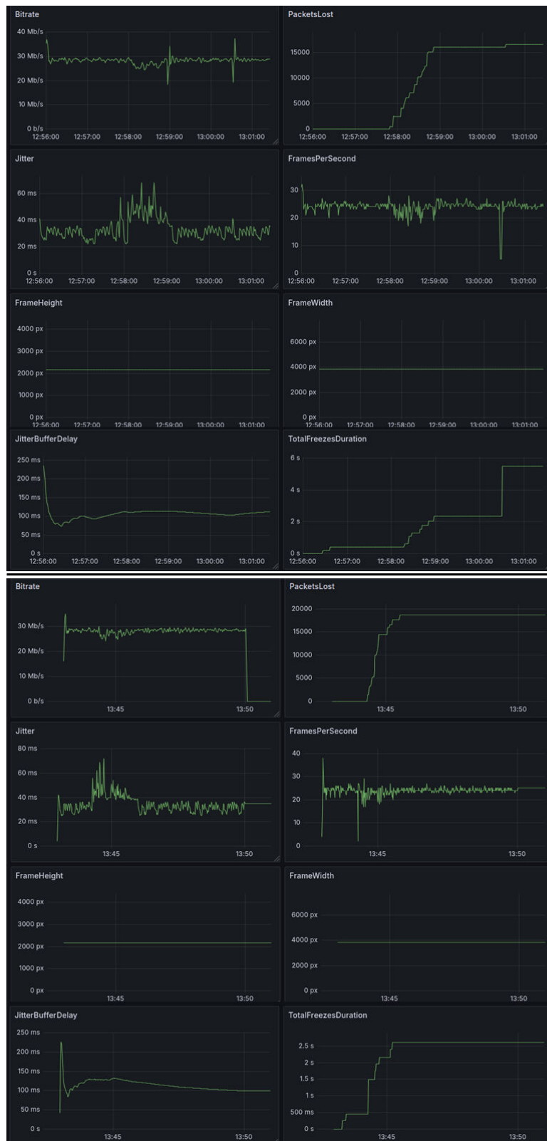
Figure 68: WebRTC session metrics collected during test run 3 (a) and 4 (b).
