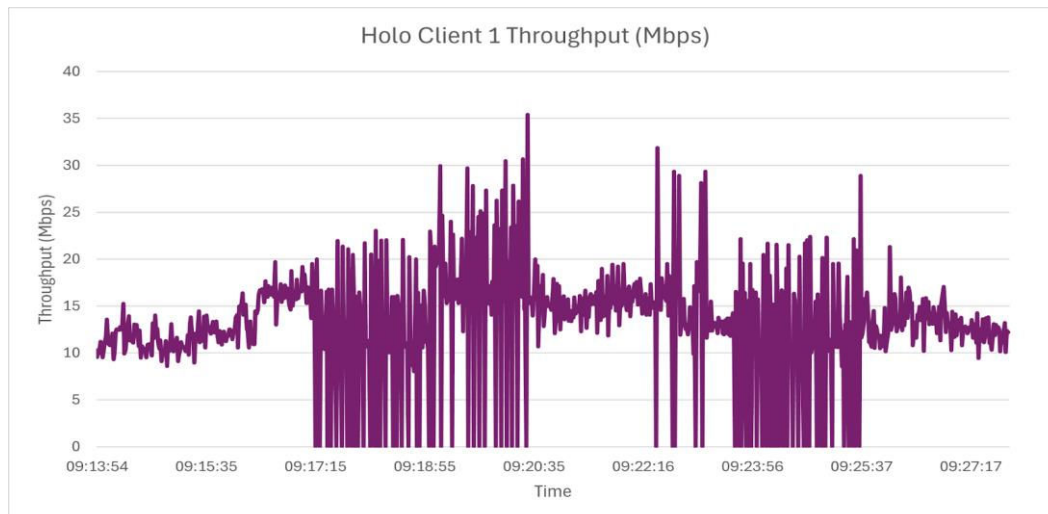
Figure 53: Uplink throughput of Holo Client 1 during the holographic session, showing sustained transmission rates over the 5G network.
