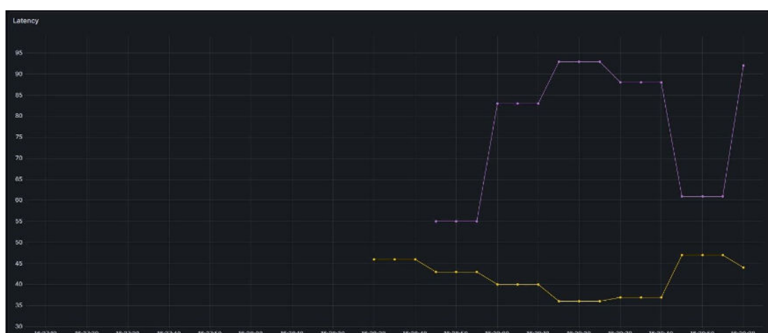
Figure 77: Latency for UE interacting with SFU in Barcelona (yellow) and for UE interacting with SFU in Madrid (purple).
