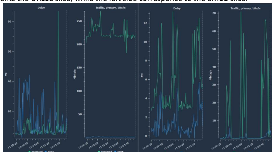
Figure 37: Throughput and latencies for both slices in scenario 2 (eMBB slice overloaded)
