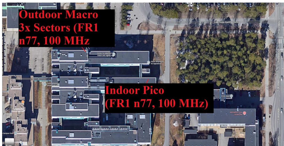
Figure 13: FR1 outdoor and indoor installation, UOULU 5GTN
