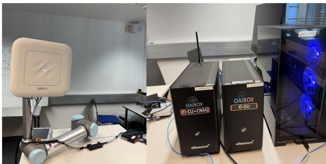
Figure 31: O-RAN FR2 (mmWave) split 7.2a setup
