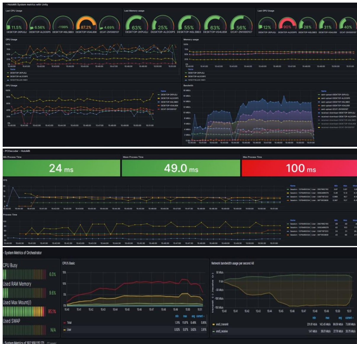
Figure 27. Grafana dashboards showing collected metrics from XR Enablers.
